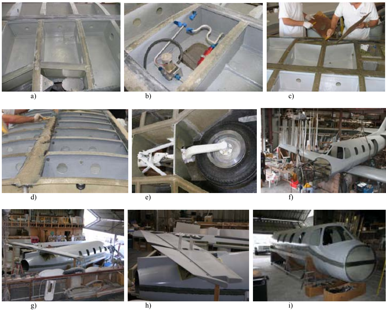
Fig. 3 a-i Production steps of aircraft Comp Air 12
